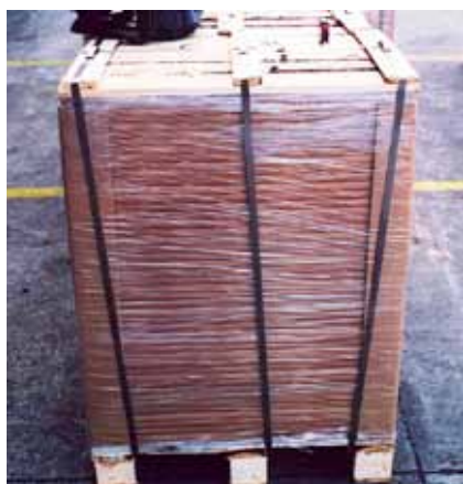
Pallet with paper in sheets with quintuple strapping. Source: Use No Hooks. p156
