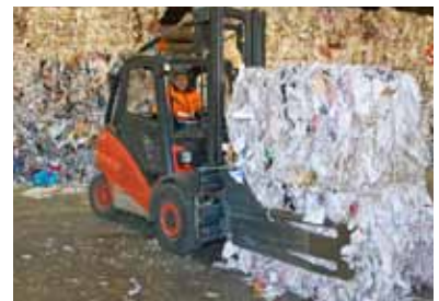
Dedicated clamps are required to handle RCP bales. Source: Ecograf..
