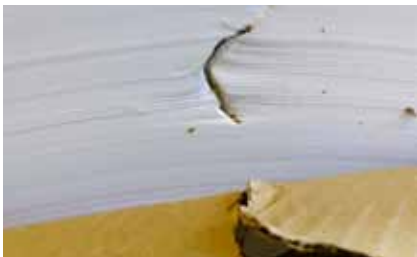
End damage from debris in floor. Source: WOCG/icmPrint.
