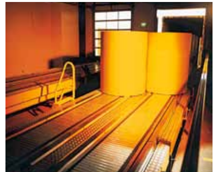
Automated truck roll unloading and conveyors. Source: Watch Next Step To Larger Roll Diameters.
