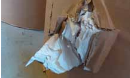
Side damage from poor clamping. Source: UPM.
