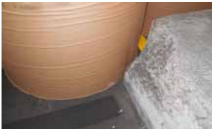
Roll damaged from collision with a wall. Source: IF P&C.
