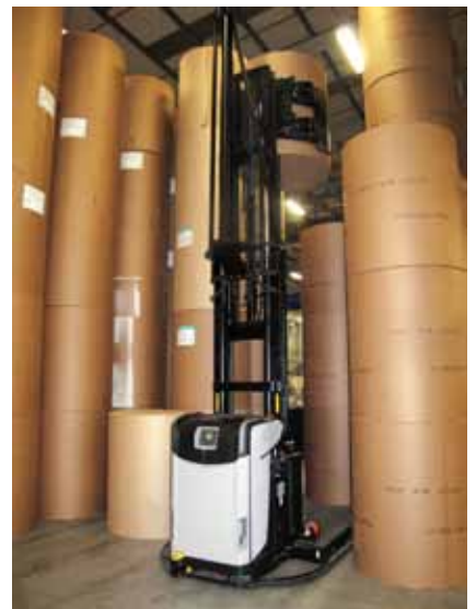
AGV automated roll handling. Source: KBA.
