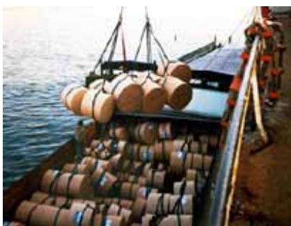
Poor stowage in general cargo vessel. Source: FMS Use No Hooks p66.
