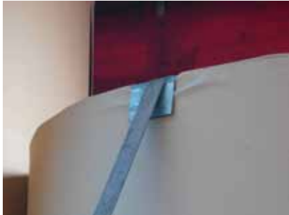
Incorrect edge protection. Source: IF P&C.
