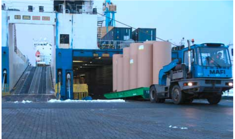
Rolls on a cassette being reversed onto the ship by a Mafi tractor. Source Intakt
