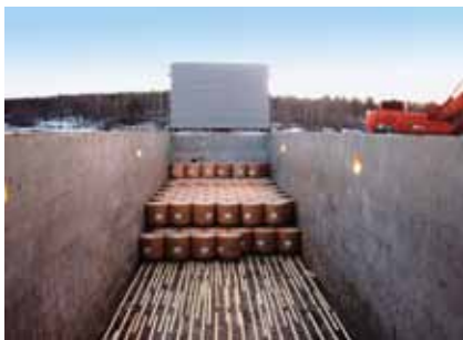
LoLo stowage and dunnage. Rolls being stowed into the hold of a LoLo vessel — the deck has timber dunnage to avoid direct contact with the deck. Source: Stora Enso.
