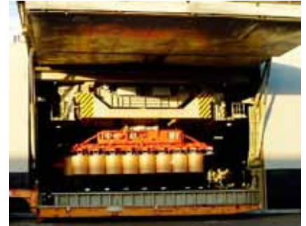
Vacuum clamp. Source: FMS Use No Hooks p 129
