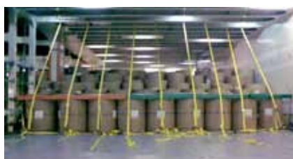
Step-down securing of StoRo cargo. Source: Stota-Enso.
