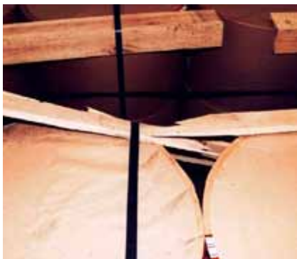
Strips of wood as edge protectors. Source: FMS Use No Hooks p 75
