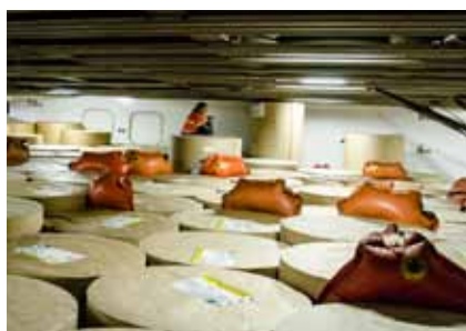
Correctly use of airbags with a StoRo cargo. Source: IF P&C.
