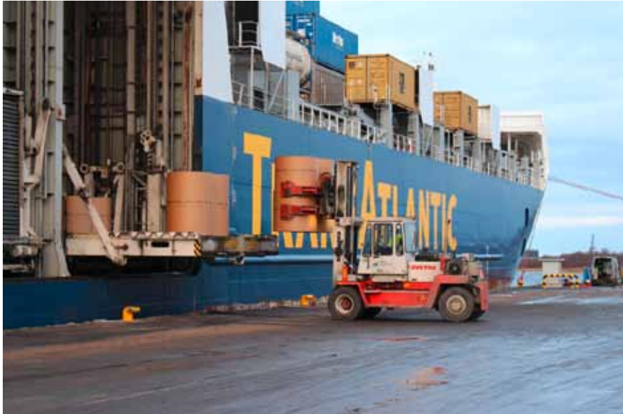
Rolls being loaded via a side port. Source: Stora Enso.
