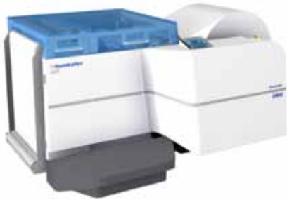
A high performance automated unwinder can handle web rolls up to 1370 mm (54") Ø weighing 1500 kg at maximum speed up to 300 m/min (1000 fpm) for web widths of 203-762 mm (8"-30"). Source: Hunkeler.
