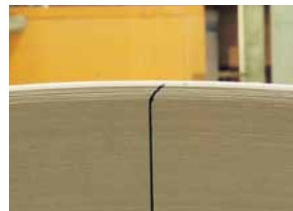
Dynamic roll expansion if wrapper removed too early. Source: WOCG/icmPrint.
