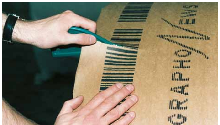
Use a roll stripper to remove the belly wrapper Source: WOCG/icmPrint.
