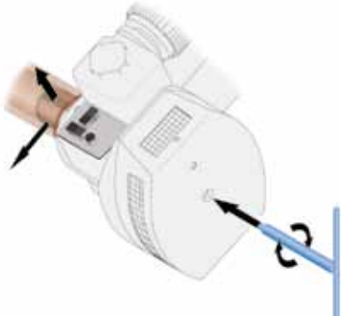
Ensure chucks are fully retracted and free of debris before loading and roll brake is switched on. Source: WOCG/icmPrint.
