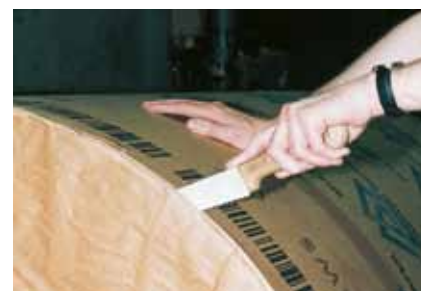
Remove end covers with a broad-bladed knife. Source: WOCG/icmPrint.
