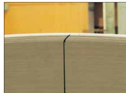
Dynamic roll expansion after wrapper removal. When unwrapped the roll acts like a released spring and will tend to loosen, putting additional tension onto splices prepared in advance. High humidity in the pressroom exacerbates the problem. Cold rolls tend to expand more when warming up. Source: WOCG/icmPrint
