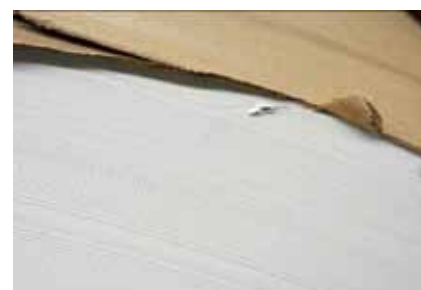
Avoid knife damage to roll. Source: ERA.
