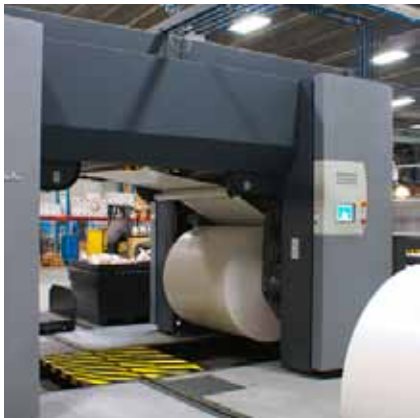
Horizontal zero speed splicer with automated roll loading. Source Goss.
